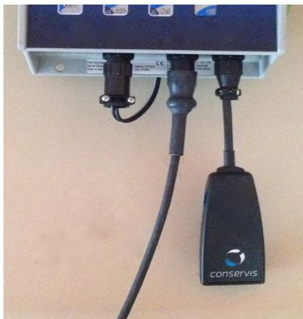
*LiveLink Bluetooth® adapter attaches to grain cart scales for automatic recording of yield data.*
